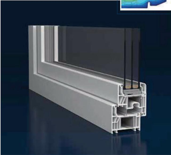
The Legend System is designed as a 6 chamber system with a 80 mm profile width. Considering the higher performance criteria in the built of the system, the profiles are engineered according to the most accurate framing .The design process is considered to include the properties for the high insulation (heat and sound), resistance, and tightness as the window performance in addition to the profile. The profiles in the systems are manufactured according to the TS-EN12608-1 standards.
