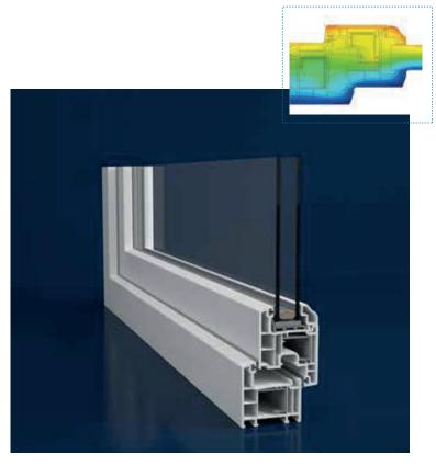
Everest Max System is 60 mm wide and designed with 4 chambers and 2 gaskets. Use of TPE gaskests has the advantage of seals on the corners and thus provides a perfect insulation.
